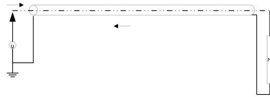
Figure 8. Schematic Diagram of Single-Ended Grounding of Shielding Layer
