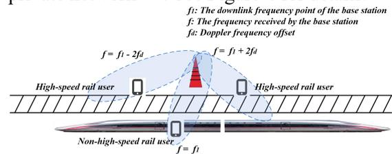
**Figure 4. Schematic of the Low-Speed User Emigration Feature**
