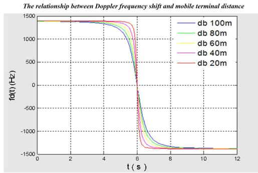
**Figure 5. Relation between Doppler Frequency Offset and Terminal Distance**
