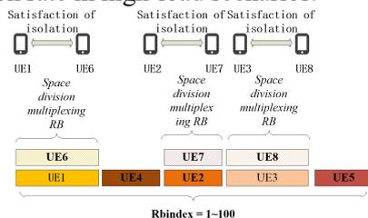
**Figure 6. Schematic diagram of uplink space division multiplexing**
