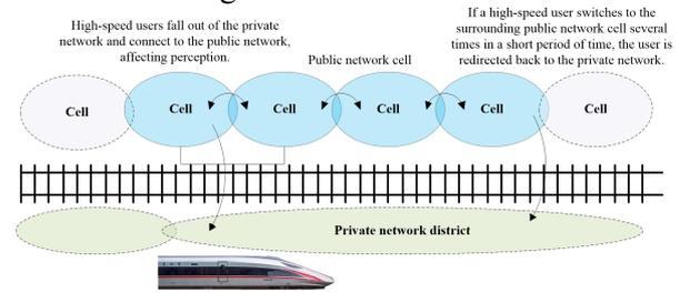
**Figure 3. Schematic of the High-Speed User Migration Characteristics**
