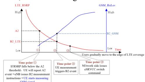
**Figure 7. eSRVCC Trigger Process**
