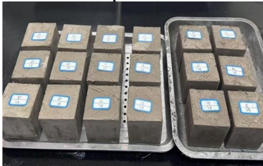
Figure 4. 70.7mm × 70.7mm 70.7mm Cubic Specimen
