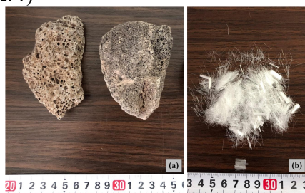
Figure. 1 Appearance of the Materials Used (A) Natural Lightweight Rocks And (B) Polypropylene Fibers Used in This Investigation
