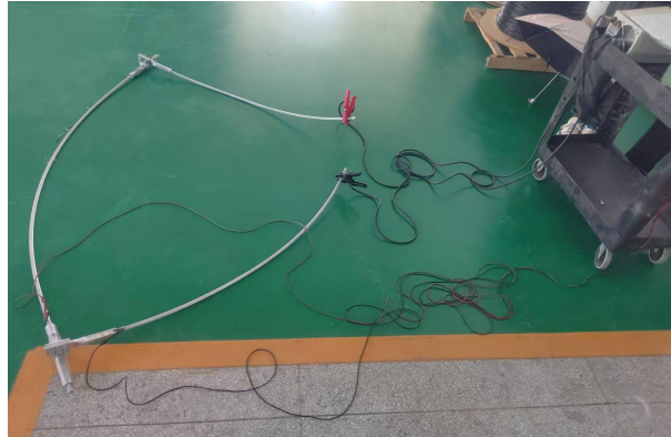
Figure 3. Measurement of Resistance before Temperature Rise for the Clamp and Equidistant Wire
