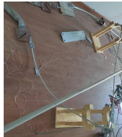
Figure 4. Layout of the Electrical Resistance Temperature Rise Test
