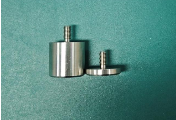
Figure 4. Physical Representation of Hammer Body Weights for Modal Testing System
