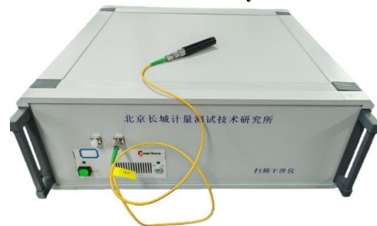
Figure 2. Photograph of the Physical Swept-Frequency Interferometric Distance Measurement System
