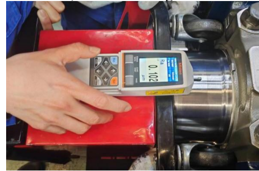
Figure 1. Actual Measurement of Roughness on the Installation Surface of the Crankshaft Rear Oil Seal
