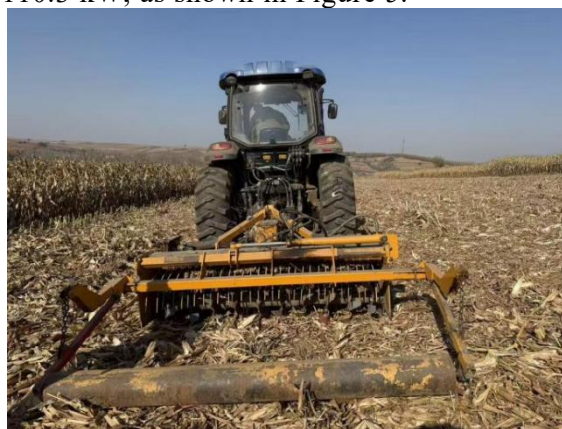
Figure 5. 1SZLYQH-202 Combined Tillage Machine for Complete Straw Return and Tillage
