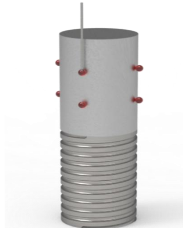
Figure 1. Schematic Diagram of Sampling Points for Installing Threaded Core Shafts on Threaded Holes
