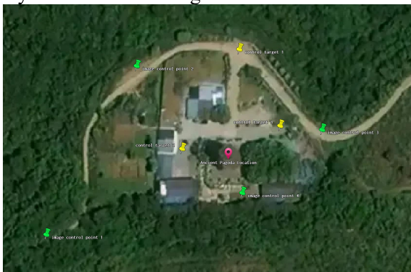
Figure 2. Distribution of Image Control Points and 3D Scanning Targets for Oblique Photogrammetry
