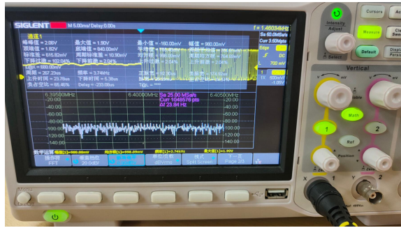
(a) Voltage Waveform of the Audio Acquisition Module
